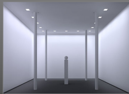
walls lit with grazing fixtures
