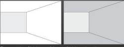
The perception of brightness of the grey field depends on the environment - in bright surroundings, an identical grey appears darker than in dark surroundings.
