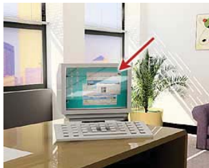
Reflected glare on computer screen from ceiling luminaries.
