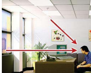
Direct glare from windows and luminaries.
