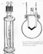
Early light bulb with a platinum filament. Although functional, its cost made the bulb commercially impractical.
