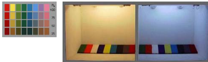
Comparing the colour appearance under different light sources (left); Test swatches under different light (right)
