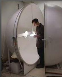
Erik is setting up a lamp for testing in the 2m integrating sphere.
