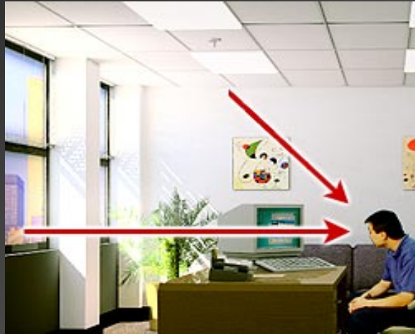
Direct glare from windows and luminaries.
