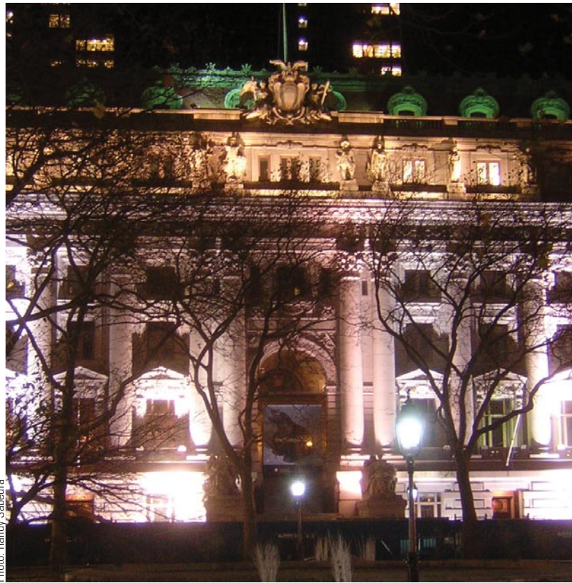
(Left, before) Prior to the relighting, the Four Continents went dark in silhouette; the building's roof had a green glow caused by mercury lamps; excessive shadows from floodlights at the base created high contrast; and the façade was bathed in a rainbow of hues from a color shift in the metal halide sources.
